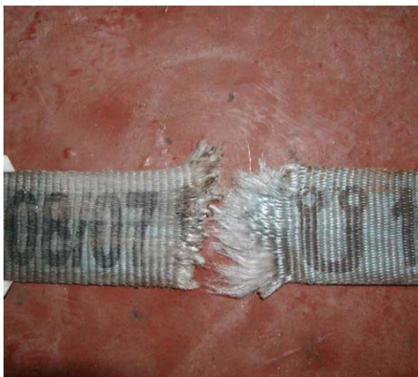
The broken sling
