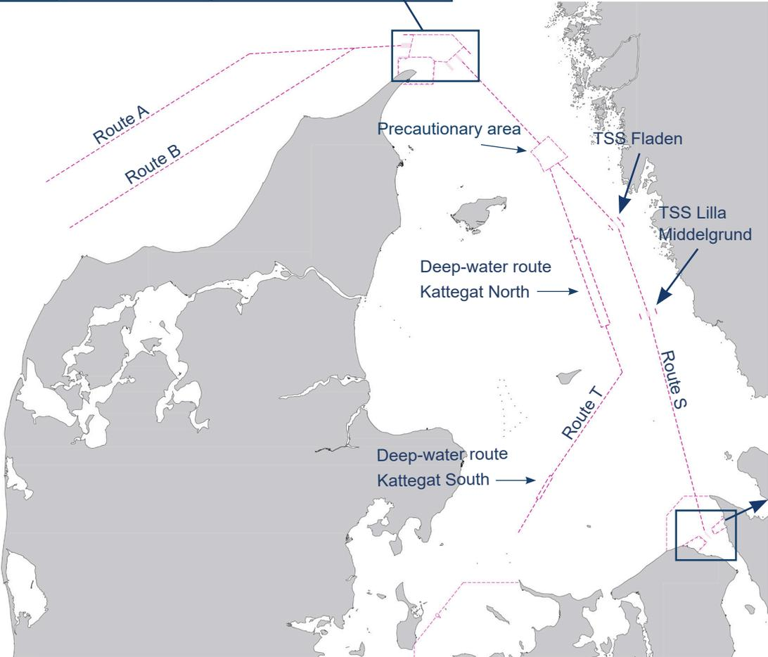
The recommended Route A holds, according to available charts, a minimum water depth of 23 metres and recommended Route B holds a minimum water depth of 14 metres.
